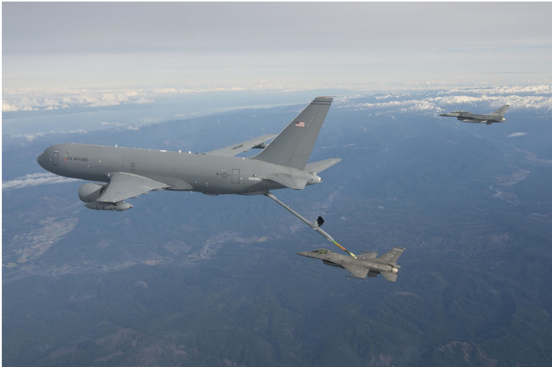
The KC-46A Pegasus performs its first-ever aerial refueling Jan. 24, 2016, passing 1,600 pounds of fuel to an F-16 Fighting Falcon. (Boeing photo/Paul Weatherman)
