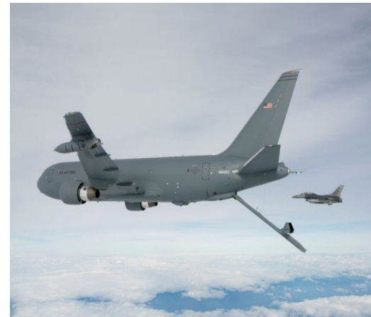
The KC-46A Pegasus Tanker deploys the centerline boom for the first time. The boom is the fastest way to refuel aircraft at 1,200 gallons per minute.
